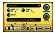
You can set loop duration by dragging the two small loop markers (LE-LS) that appear on the timeline when you enable loop play. The loop duration will be highlighted in green.
