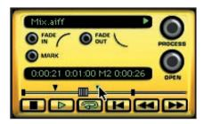
You can stop and restart playback by clicking on th transport buttons. By dragging the slider (even during playback) you'll be able to forward through your mix.
