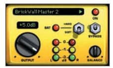
The output level is indicated by the program peak meters consisting of three LEDs. They will show you when your master reaches -3 dB, -1 dB, and 0 dB levels.
