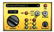
With the OUTPUT control you can set the MASTER LEVEL of your mix. The output section has to do the job of fitting the ultra-high digital resolution of the internal T-RackS
